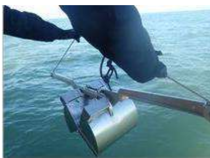
Figure 4 : Benne Van-veen (0.1m 2 )
